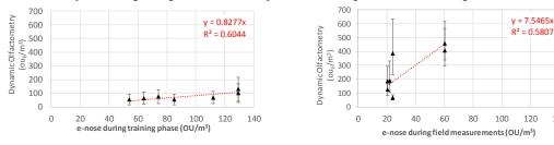
Figure 8. Correlation between OU/m<sup>3</sup> values obtained by the dynamic olfactometry and the e-nose.
