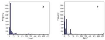
Figure 6: Different probability distributions of OU/m<sup>3</sup> measured by MSEM-32 e-nose, in correspondence of SSE wind and calms (a:Waste landfilling on; b: Waste landfilling out).
