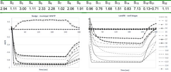
Figure 2: Response of MSEM32 e-nose sensors to the odour classes associated to different sources. There are shown only the sensors with a high value of  $\Delta R/R$ : the sensor response for each time point is calculated as  $(R_t-R_0)/R_0$ , where  $R_0$  is the initial resistance value. Hence the initial datum has  $\Delta R/R = (0-R_0)/R_0=0$ . The time 0 sec corresponds to the start of the odour sampling by the e-nose.
