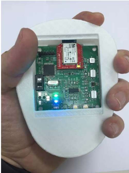
Figure 1: Prototype of the electronic nose
