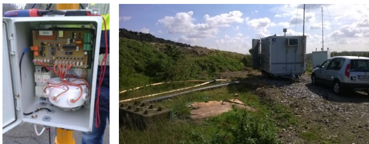
Figure 2: illustration of the sensors-array device (left) and of the mobile laboratory-installed in MSW-1- (right)
