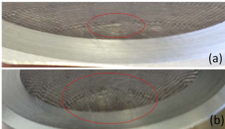
Figure 3: Surface modification (a) and final breakage (b) of the sample during the abrasion testing.
