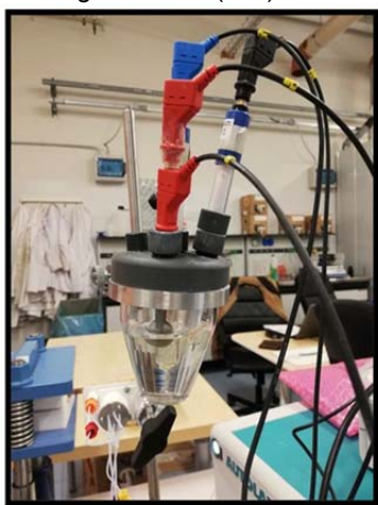
Figure 2: Electrochemical cells used for corrosion tests.
