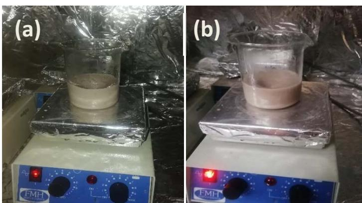
Figure 1: (a) ZnO before and (b) and after the addition of Ag<sub>2</sub>S during synthesis in dark
