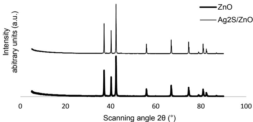
Figure 2: XRD pattern of ZnO and Ag<sub>2</sub>S/ZnO catalysts synthesised by sol-gel method
