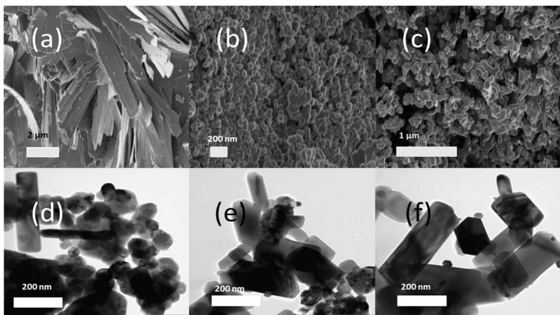
Figure 3: SEM image of (a) precursor ZnO. (b) pure ZnO. (c) Ag<sub>2</sub>S/ZnO. TEM image of (d) precursor ZnO. (e) Pure ZnO. (f) Ag<sub>2</sub>S/ZnO
