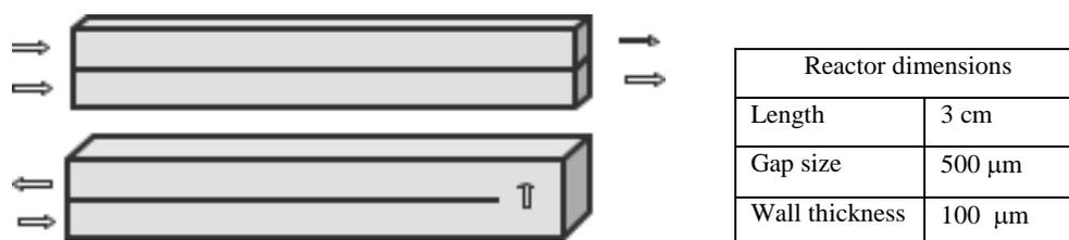
**Figure 1:** Schematic of straight channels (top) and U-bend (bottom) for representational purpose. Arrows denote the flow direction.
