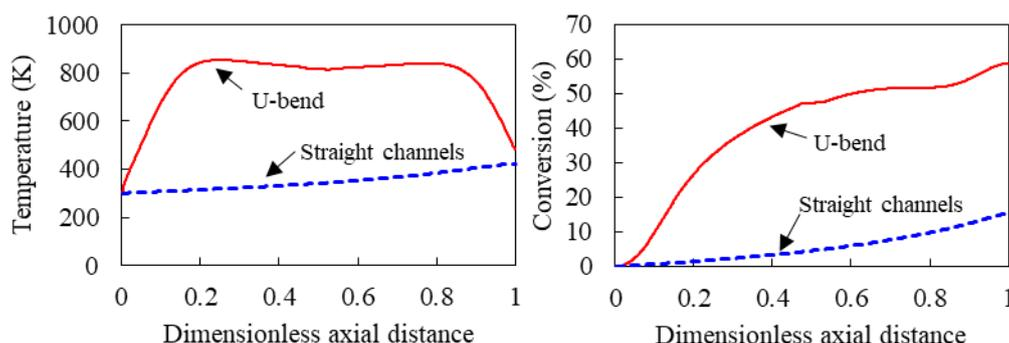
**Figure 2:** Temperature (left) and conversion (right) patterns for both reactors along the axis.
