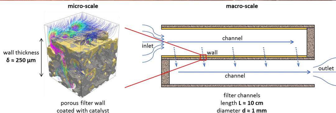
**Figure 1.** Multi-scale model of catalytic monolith filter. Left: 3D reconstructed wall (grey = substrate, yellow = coated catalytic material) with calculated flow field (streamlines) [4]. Right: Scheme of the filter channels simulated with full-scale 1D+1D model [2].
