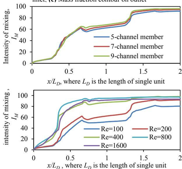
**Figure 3.** Mixing intensity plots: (a) Variation in  $I_M$  with  $Re$  for different threading configurations; (b) Variation of  $I_M$  along the length of the reactor at different  $Re$
