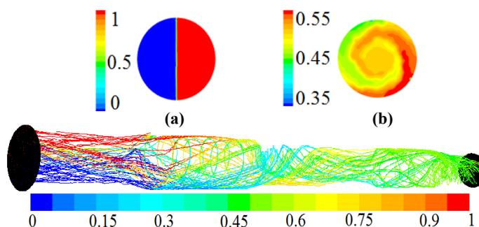
**Figure 2.** Results for 7-channel member,  $Re=200$  (a) Path lines colored with tracer mass fraction; (b) Mass fraction contour on inlet; (c) Mass fraction contour on outlet
