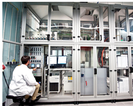
Fig. 1: Pilot scale fixed bed reactor for spatially resolved measurements.
