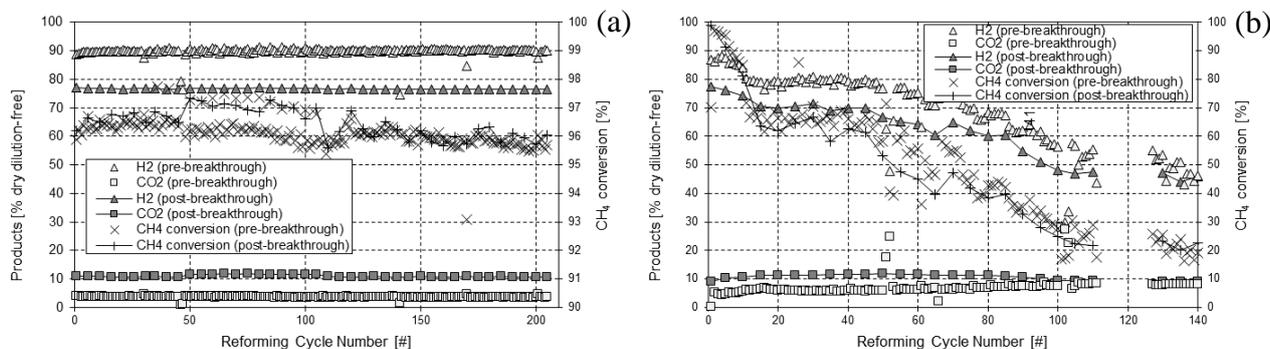
**Figure 1.** Multicycle SESMR/regeneration tests on CaO15Ni(N)10, with mild (N<sub>2</sub>, 850 °C) (a) or severe (CO<sub>2</sub>, 925 °C) regenerations.
