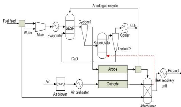
**Figure 1.** Schematic diagram of the bio-oil sorption enhanced steam reforming and SOFC integrated process.
