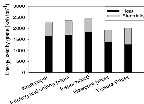
**Figure 2.** Heat and power demand of different paper grades in the paper industry [6].
