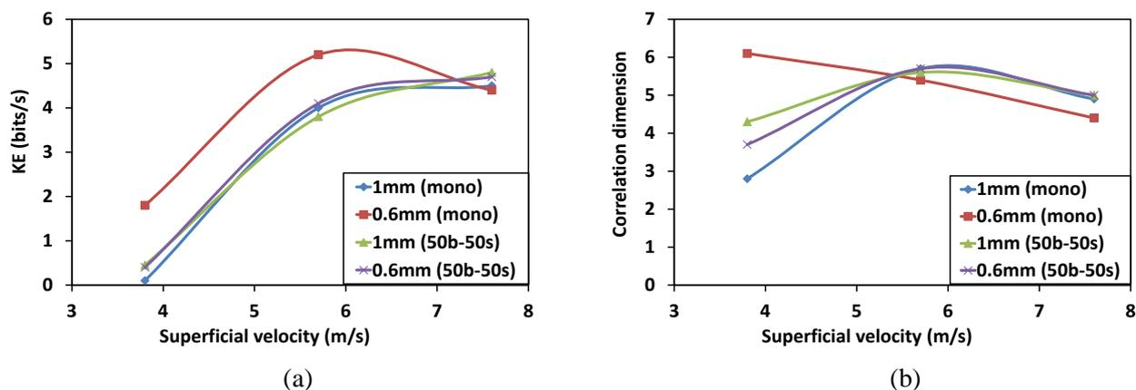
Figure 1. Kolmogorov entropy and Correlation dimension of different composition with superficial velocity
