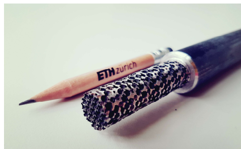
Figure 1. Structured reactor used during the experimental activity. A part of the outer wall was removed for visualization purposes.
