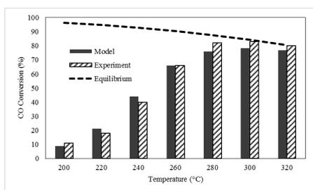
**Figure 1.** Comparison of CO conversions obtained from experiments [1] and mathematical model.
