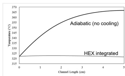
**Figure 2.** Temperature distribution along the centerline of the reaction channel in case of absence and presence of cooling.
