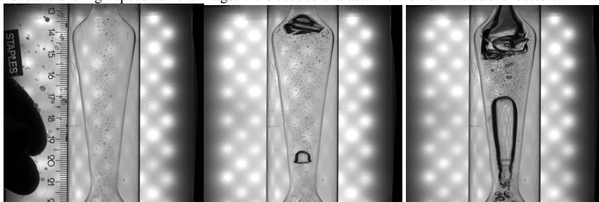
Figure 1. Gas and liquid flow in a compartment of the pulsating flow column reactor.
