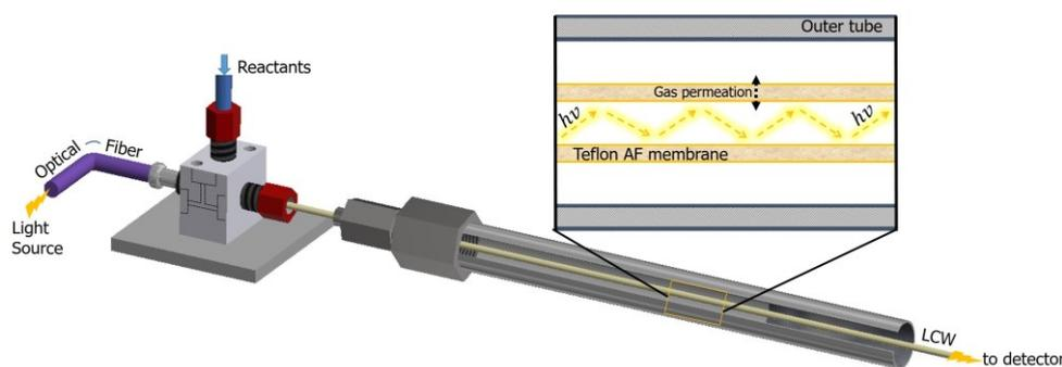
Figure 1. Schematic LCWM setup for *in situ* sensing and permeation using a Teflon AF tube (not to scale drawing)
