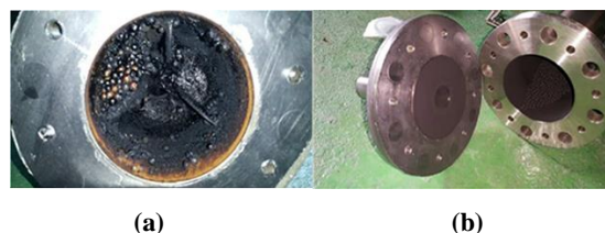
Figure 3. Char foaming and agglomeration of lignin with fluid bed reactor, and rotary kiln reactor
