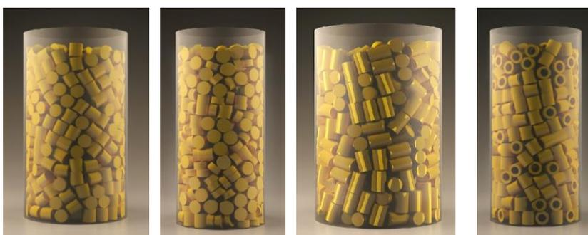
**Figure 2.** Random packings of particles of different shapes with  $d_t/d_{pv}=7$
