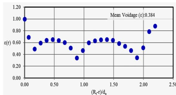
**Figure 1.** Radial void fraction profile of rasching ring packing with  $d_t/d_{pv}=5$ , computed using polygon-based radial method
