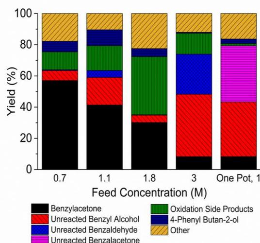
**Figure 2.** Yield of the various reaction products from the multistep flow synthesis of benzylacetone in flow from four different inlet concentrations of benzyl alcohol (0.7, 1.1, 1.8 and 3 M) and also in the one pot synthesis using 1 M feed. The desired final product, benzylacetone is shown in black.
