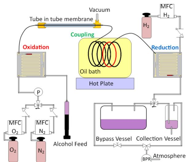
**Figure 1.** Experimental set-up for the multistep synthesis of benzylacetone and 4-(4-methoxyphenyl)butan-2-one. The red sections in the reactors represent the catalyst packed bed, MFC stands for mass flow controller, BPR for back pressure regulator and P for pressure sensor.
