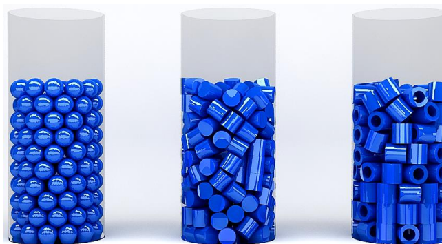
Figure 2. RBD-simulated structures of (a) spheres, (b) equilateral solid cylinders and (c) rasching rings, with d_t/d_{pv} = 5 .
