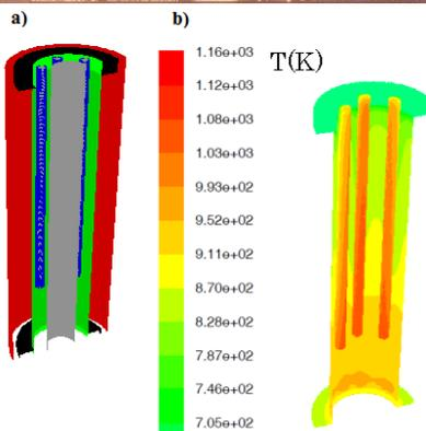
**Figure 1.** - a) Control volume of the 3D-CFD model; b) Temperature profile on the control volume
