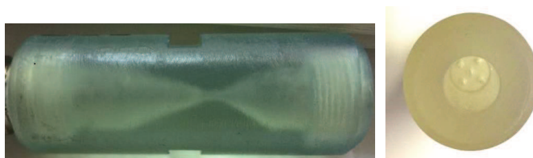
Figure 2. Pictures of the Venturi tube and orifice plate devices used for the experiments
