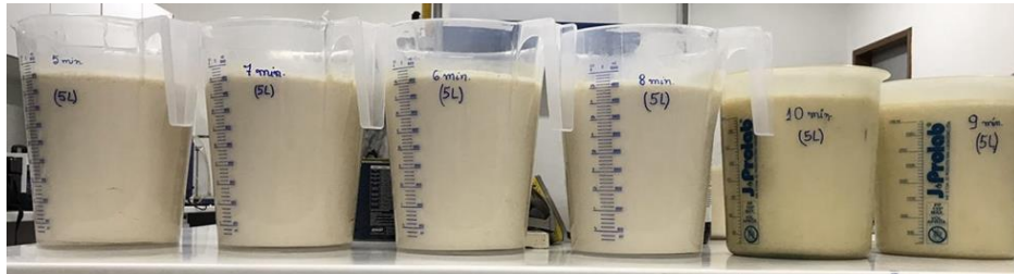
Figure 3: Biodetergent production tests to assess physical parameters in volume of 4 and 5 liters, after 96 hours of rest
