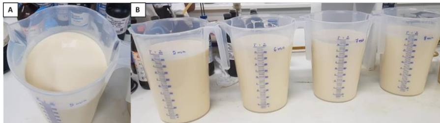
Figure 1: Biodetergent production tests to assess physical parameters for volumes of 4 and 5 liters. (A) aspect of the formulation right after production. (B) production tests for some investigated stirring times
