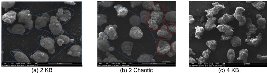
Figure 7: 40X SEM images of (a) 2 KB and (b) 2 chaotic under 50rpm / 60 °C / 5% with (c) 4 KB. Blue regions showing more fines, red ovals showing crushed granules and the red rectangle showing evidence of granule breakage
