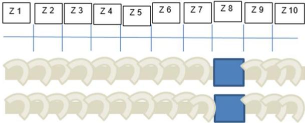
Figure 3: Schematic of co-rotating screw configuration showing mixing zone at zone 8 (z 8)
