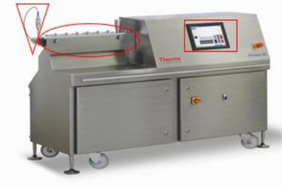
Figure 2: External view of Pharma 16 twin screw co-rotating extruder; inverted triangle with the temperature probe; oval shape is the extruding barrel section containing the twin screws; the rectangular shape is the control and display unit (ThermoFischer Scientific)
