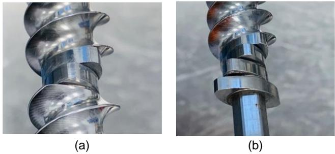
Figure 4: Kneading element configuration; (a) 2 KB and (b) 4 KB.
