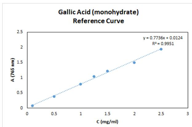
Figure 1. Reference curve of pure gallic acid (monohydrate).
