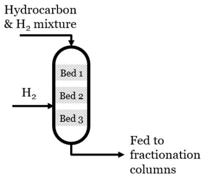
Figure 1: Hydrodesulfurization reactor with three catalyst beds.
