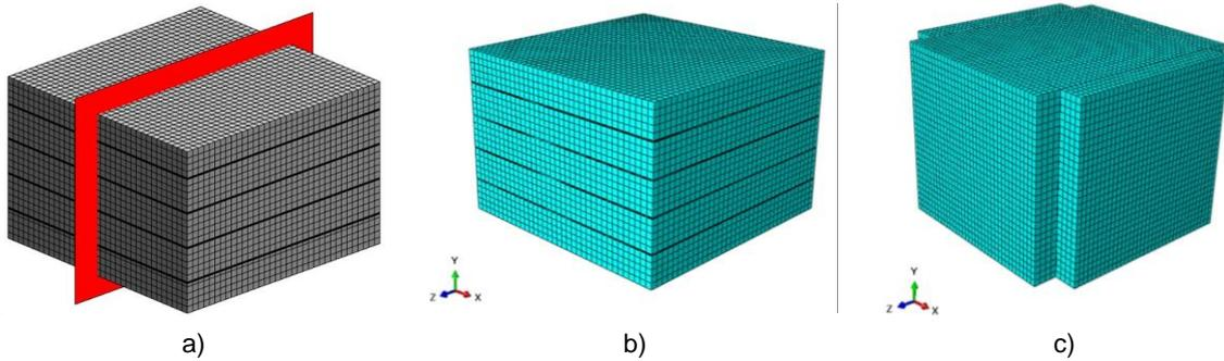
Figure 2: Discretization of the isolator into 3D finite differences (a), into 3D finite elements (b) and into 3D finite elements with steel mould (c).
