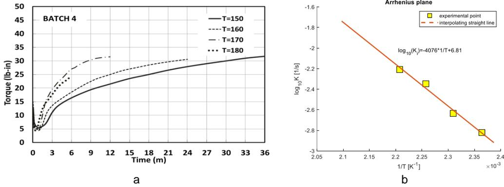
Figure 1: a) Rheometer curves obtained for batch 4B. b) experimental determination by linear best fitting of the reaction kinetic constant for the rubber blend.
