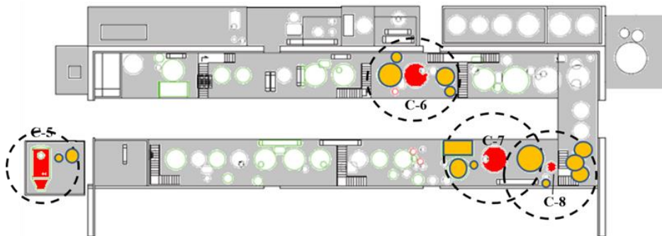
Figure 5: Graphical representation of SW&HI damage area, before (top) and after (bottom) implementation of control measures, in department C (units containing flammables with greater than 5 SW&HI are depicted in red, others in yellow)
