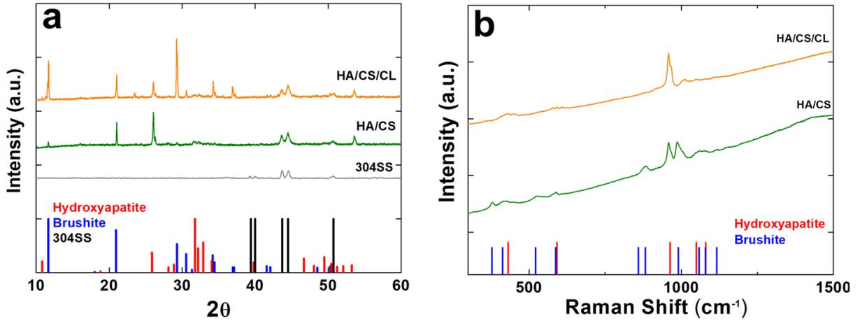
Figure 2: a) XRD patterns of HA/CS and HA/CS/CL obtained after 24 h at 50°C. b) Raman spectra of HA/CS and HA/CS/CL obtained after 24 h at 50°C.
