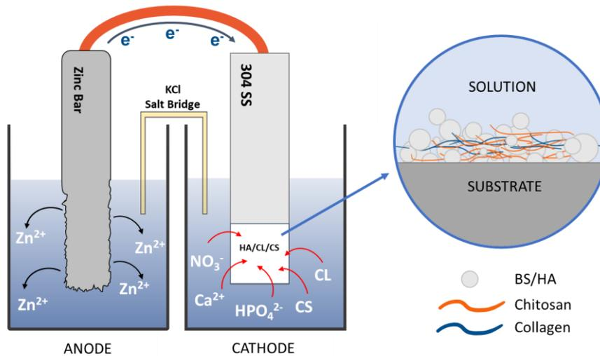
Figure 1: Separate cells system for galvanic deposition process
