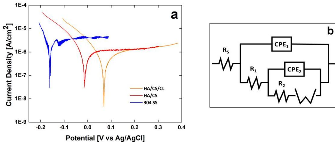
Figure 4: a) Tafel plots measured in SBF solution for HA/CS and HA/CS/CL coated samples obtained by galvanic deposition. For comparison, the plot relative to uncoated 304SS is also reported. b) Equivalent circuit used for impedance fitting
