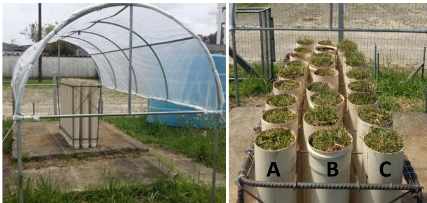
Figure 1: Test condition of columnar field reactors with grass cover detail, being row "A" reactors without contamination, row "B" reactors with contamination of pre-treated effluent and row "C" reactors with contamination of effluent without pre-treatment. Photo: The authors
