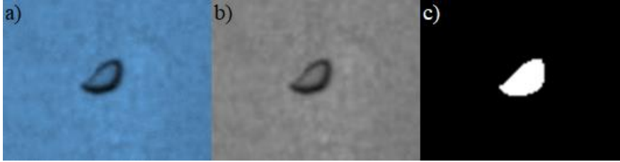
125 126 Figure 2: Selected stages of image processing; a) colour image, b) grayscale image, c) binary image
