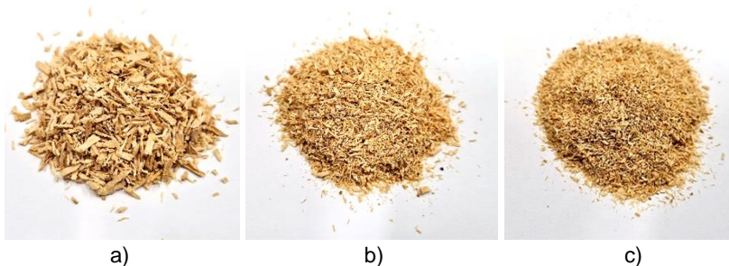
Figure 4: Particle shape after milling the raw material on a screen sieve with squared openings (4HR), with dimensions a) 6x6mm, b) 4x4 mm, c) 2 x 2mm.
