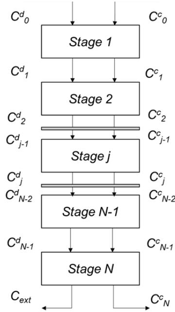
Figure 1. Electrodesalination System operating in N stages
