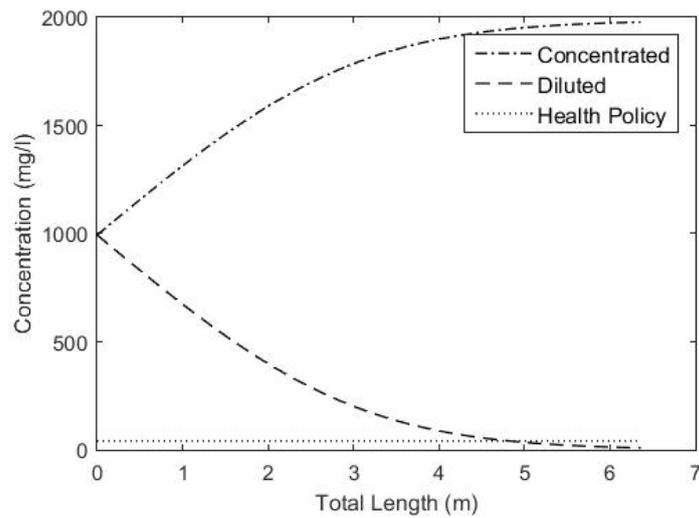
Figure 3. Diluted and Concentrated flows profile throughout the ED system.
