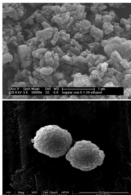
Figure 2: small (top) and large ZSM-5 crystals (bottom)
