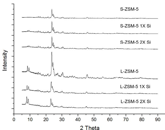
Figure 1: XRD patterns of ZSM-5 samples
