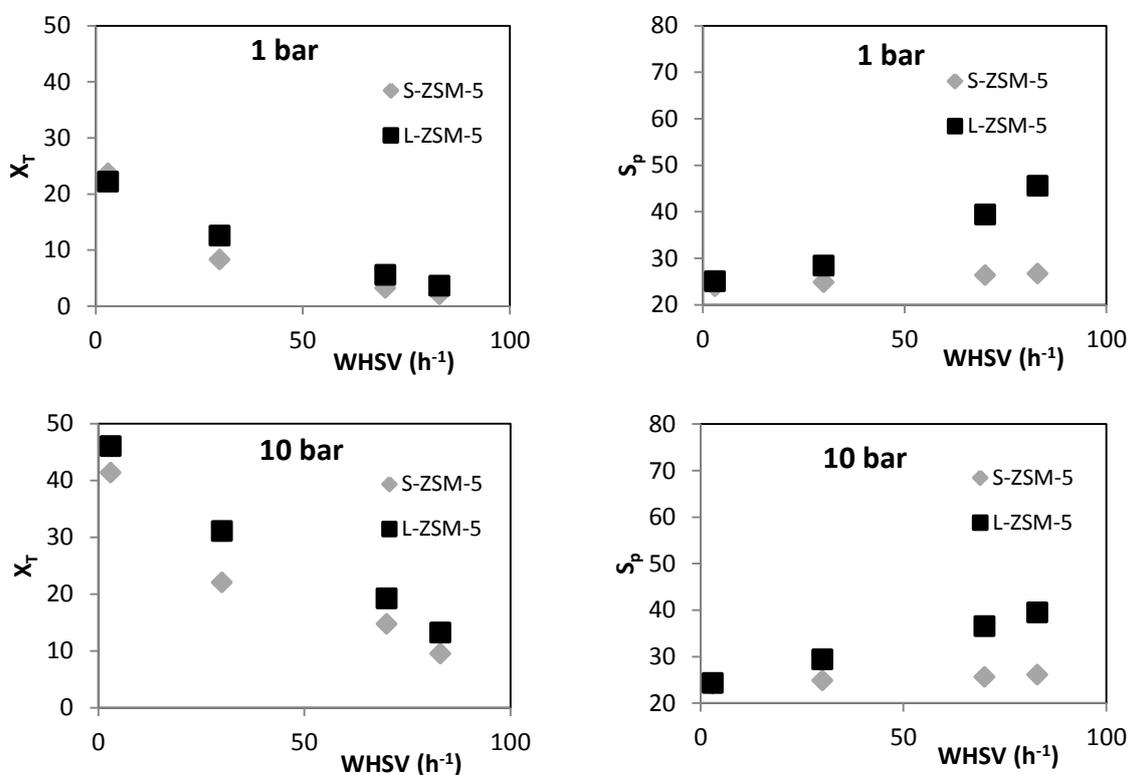
Figure 3: Effect of crystal size on toluene conversion and *p*-xylene selectivity at 1 and 10 bar
