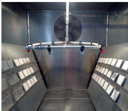
Figure 1: Weathering chamber with samples before starting the last 20 cycles.
