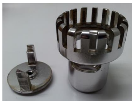
Figure 3: Left: the rotor and the stator of the T 50 Ultra-Turrax® - IKA mixer. Right: experimental values of the product distribution X_s versus energy dissipation rate. X_{s,\text{eff}} is based on the process efficiency, Figure 5b.
