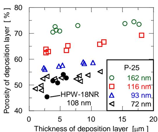
Figure 6. Effect of particle size on porosity of particle deposition layer.
