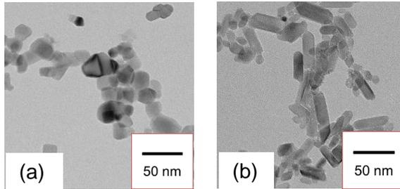
Figure 1. SEM images of (a) P-25 NPs and (b) HPW-18NR NPs.
