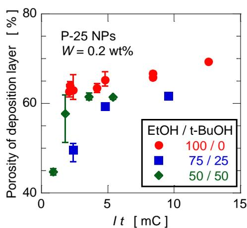
Figure 8. Porosity of particle deposition layer prepared by EPD from P-25 NPs in mixture solvents.
