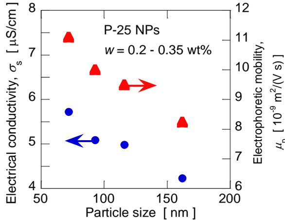
Figure 3. Effect of particle size in EPD sample suspension on electrical conductivity of suspension and electrophoretic mobility of particles.
