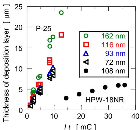
Figure 5. Thickness of particle deposition layer prepared by EPD from suspensions with various particle sizes.
