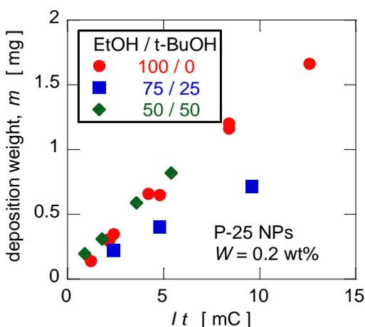
Figure 7. Particle weight deposited by EPD from P-25 NPs in mixture solvents.
