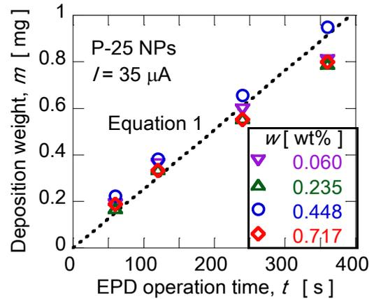
Figure 2. Effect of water content on particle weight deposited by EPD and calculated by Equation (1).
