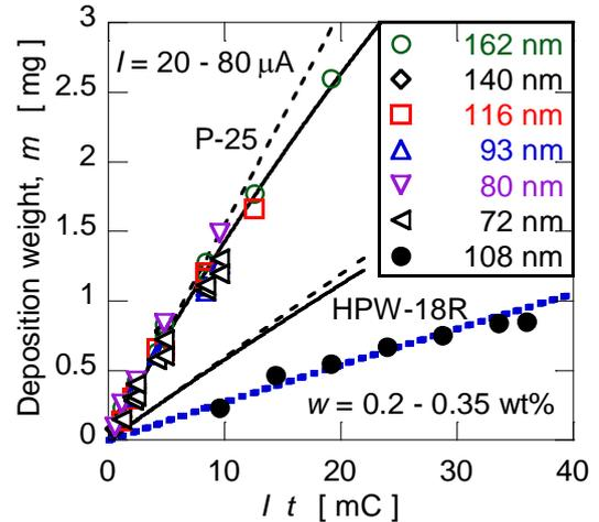
Figure 4. Particle weight deposited by EPD from suspensions with various particle sizes.
