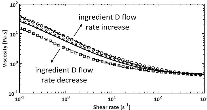
Figure 3: Rheological behavior of the detergent at different process conditions.
