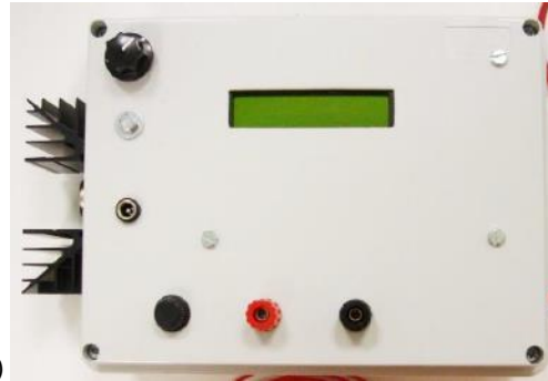
Figure 2. a) Ceramic heater b) Automatic power controller, used for the determination of the heat exchange coefficient.
