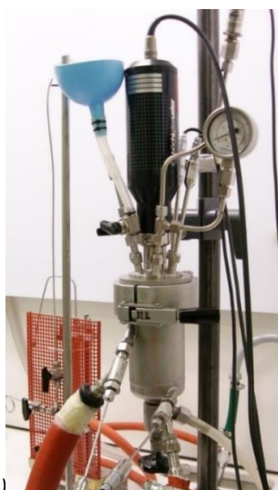
Figure 1. a) Calorimetric reactor by BüchiGlasUster. b) Thermocryostat by Huber used for the determination of the heat exchange coefficient.
