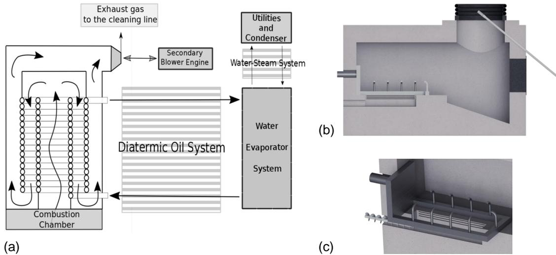
Figure 1: Scheme of the (a) combustion system, (b) chamber and (c) secondary air injection.
