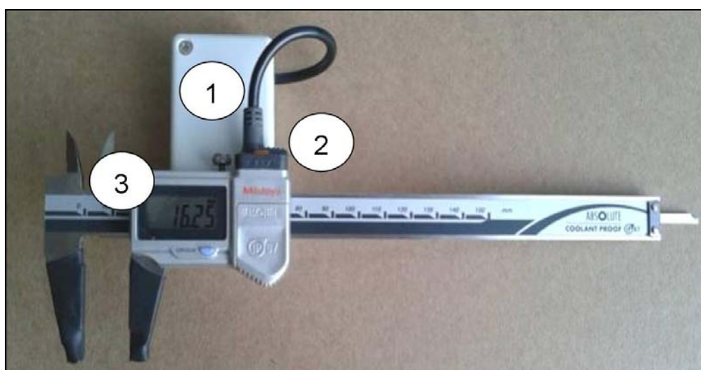
Figure 2. Digital Caliper with onboard datalogger (Calibit). 1Datalogger; 2Recording Button; 3 Data display
