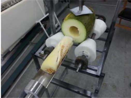
Figure 9a. The first melon scoop operation for removing internal seed part.
