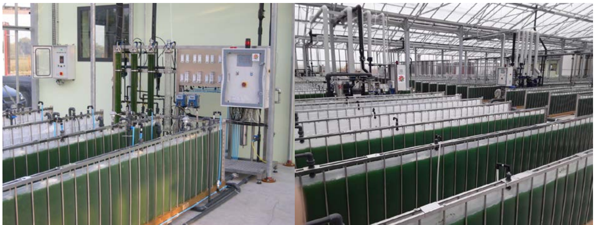
Figure 1 – Inoculum area (left) and GWP ® -II reactors under a greenhouse for algal mass cultivation (right).
