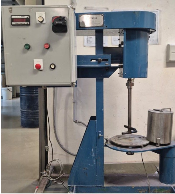
Figure 1. Laboratory scaled vertical stirred media mill, showing the stirrer and bucket beside it. Taken at the University of Cape Town.
