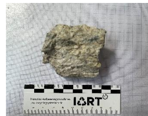
Figure 4 Single particle testing (left: before the test, right: after the test). Tests on (a) zinnwaldite ore (10 Imp-90J) (b) lepidolite ore (150 Imp-90J) and (c) petalite ore (15 Imp-90J).
