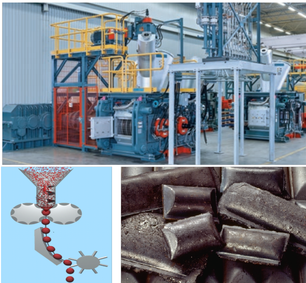
Figure 6: DRI-HBI application of roller presses
