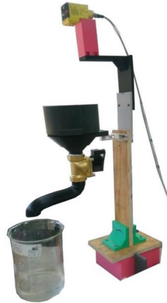
Figure 6. Assembled concept design of the density meter.
