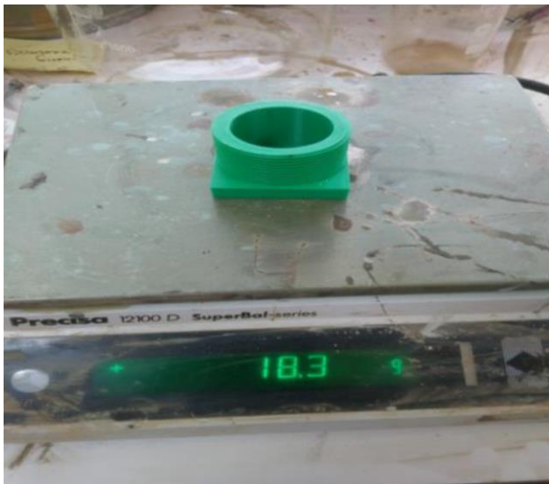
Figure 5. The mass of the object measured with a calibrated scale
