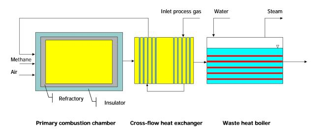
The student must design the three process units. It is necessary to quantify the geometrical dimensions of each process unit as well as its inlet and outlet streams in terms of flowrate, compositions, and temperature. Any additional information/dimension/quantity necessary for the measuring of the process/plant is welcome. Finally, the student should provide and discuss the assumptions, and possible simplifications taken to design the plant.
