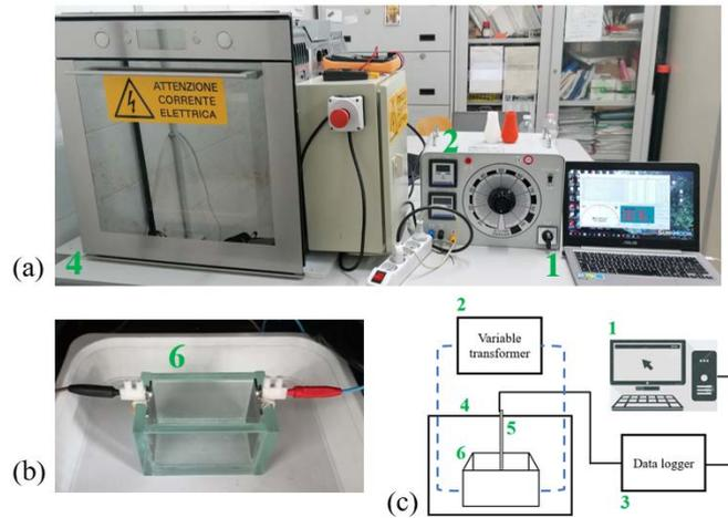
Figure 1: Pictures of the adopted instrumentation: (a) assembly of the MEF heating equipment, showing the (1) data acquisition system, (2) the variable transformer and (4) the insulated chamber. (b) Detail of the (6) MEF cell with the electrodes. (c) Schematic diagram of the experimental setup representing the insertion of (5) the thermocouple into the cell.
